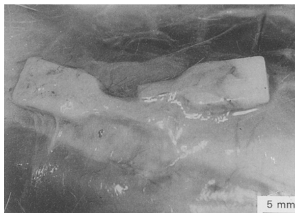
Figure 3 Photograph of a broken dumb-bell in situ in the back of a rat.
